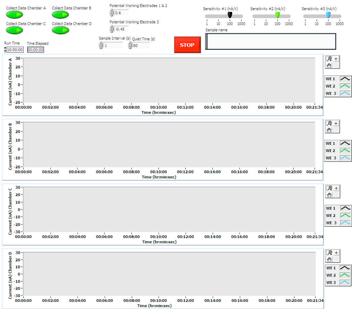
Figure 16. User interface of the LabVIEW program written for the multipotentiostat for use with the MAMP
