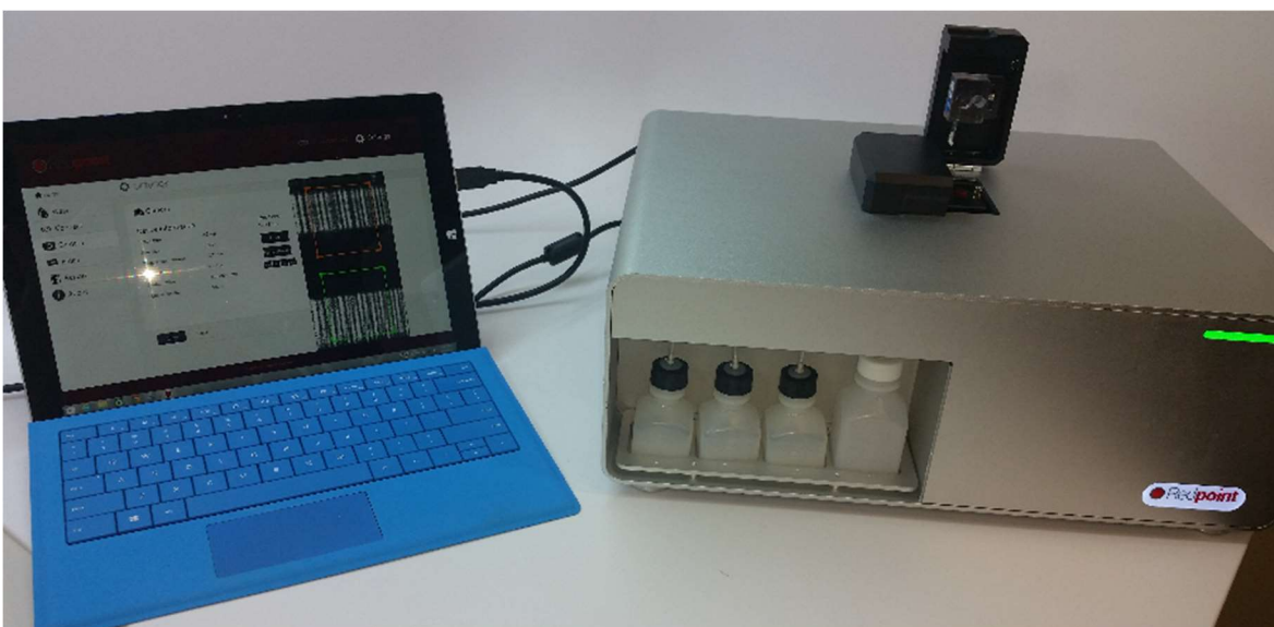
Fig. 9.1 The Redpoint Platform developed in collaboration with Biotex, Inc, represents a fully functional prototype benchtop interaction photometer based upon the compensated interferometer.
