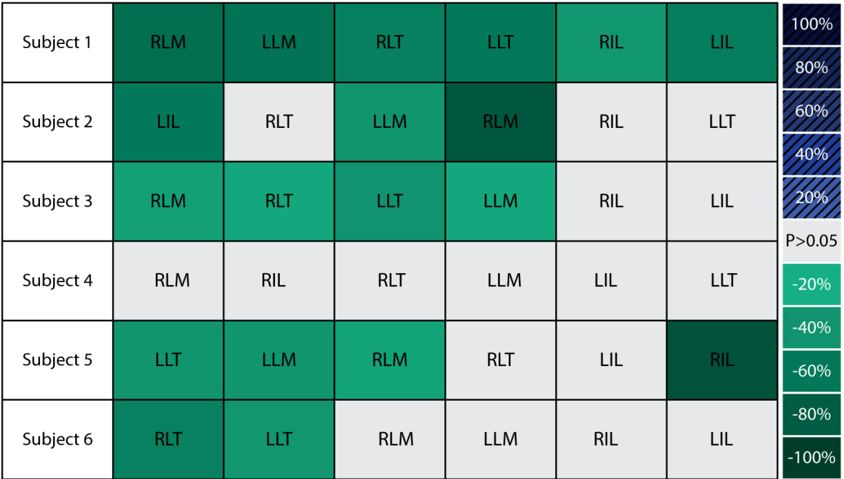
Figure 3.6: Individual muscle responses to exosuit vs. muscle fatigue rate. This shows Case I results (from Table 3.2) reorganized such that muscles are ordered from left to right, where left is the fastest (and right is the slowest) rate of fatigue during control trial A1. Significant decreases (and increases) in MDF slope are denoted by green (and blue) shading, where darker shades indicate larger magnitudes of change. Non-significant changes are denoted by light gray shading. Muscles that fatigued the fastest during control trial A1 tended to show significant reductions with the exosuit intervention, depicted by the higher density of green boxes on the left (and gray boxes on the right).
