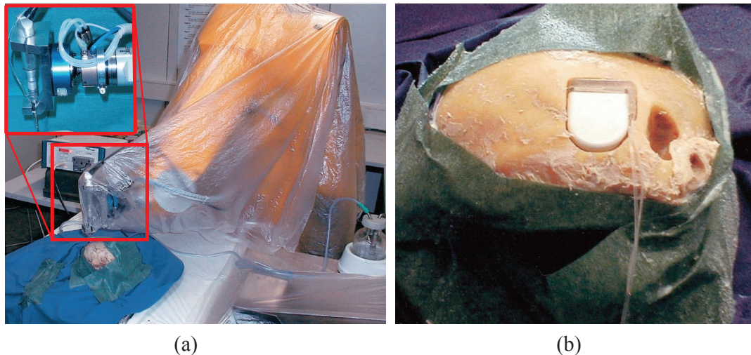
Figure 1.4: (a) Force-controlled robot for milling a cavity in temporal bone for a CI receiver (developed by Federspil et al.) with an inset showing closeup of the surgical drill end-effector and force sensor. (b) The milled out cavity with the CI receiver placed into it (images from [1]).
