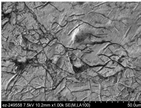
Figure 5.2: Polished {}^6\text{LiInSe}_2 ceramic under 1000X magnification with a 10.2mm working distance.
