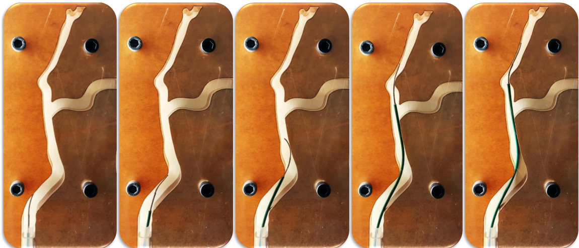
Figure 4.32: Video snapshots of autonomous catheter insertion and steering in 2D ICA model
