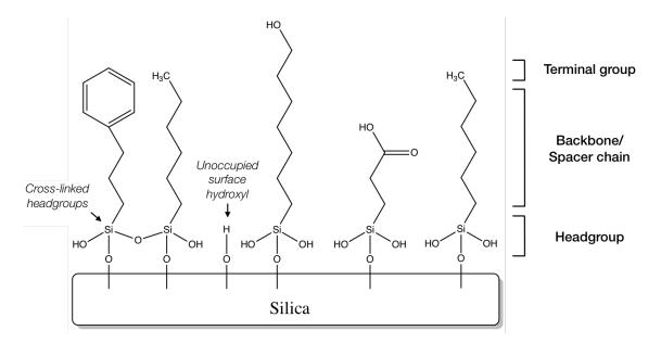
Figure 1.1: Visualization of monolayer thin films studied with optimizable components, *e.g.*, terminal group, backbone, backbone chain length, degree of crosslinking, and film composition.
