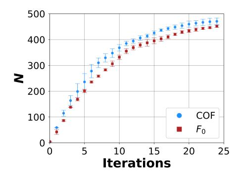
Figure 4.4: The amount of systems in the top 500 systems, ranked by either their simulated COF properties or  $F_0$  properties, that is captured by a hypothetical iterative integration of ML model to the high-throughput screening process.
