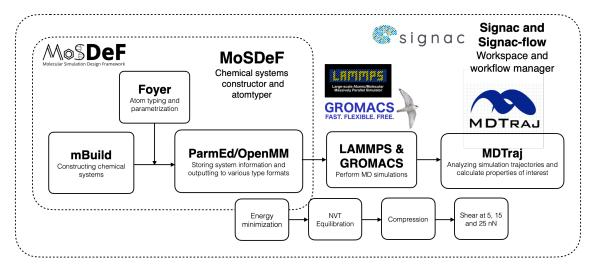
Figure 2.3: High-throughput screening workflow utilizing all open-source software. Specifically, the MoSDeF software suite is utilized to automatically perform system initialization, while GROMACS and LAMMPS are used to perform the molecular dynamics simulation, whose results are analyzed with MDTraj; the workspace and workflow as a whole is managed by signac and signac-flow.
