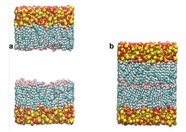
Figure 2.1: Snapshot of dual-monolayer system (difluoro-terminated on both top and bottom monolayer) during the energy minimization (a) and shearing (b) stage
