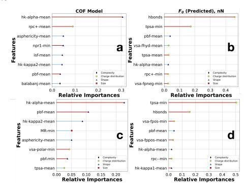
Figure 4.2: Feature importance of Summers *et al.*, model for (a) COF and (b)  $F_0$  in comparison with those of ML models trained with data generated from this study for (c) COF and (d)  $F_0$
