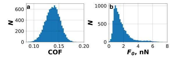
Figure 3.2: Distribution of (a) COF and (b)  $F_0$  for systems considered in this study, obtained from MD simulations
