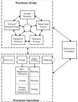
Figure 4: Framework for warehouse design and operation problems (Manzini et al., 2011)
