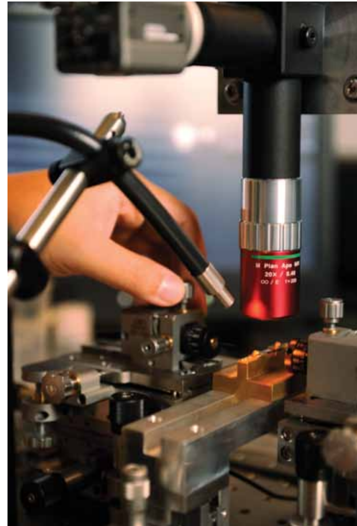
This high-precision optical measurement system allows light to couple from an optical fiber into a silicon waveguide sample located under the red microscope objective lens.
